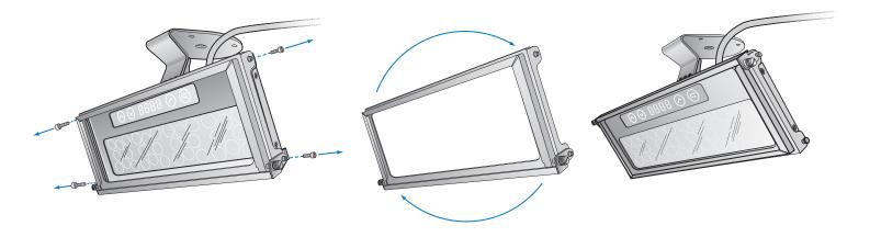
2. Loosen the two captive thumbscrews located on the upper edge of the accessory holder, and pivot the top of the accessory holder back to expose the slot.
