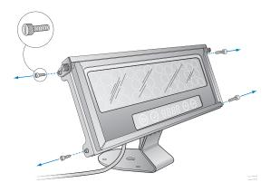
2. Remove the accessory holder from the fixture housing.
