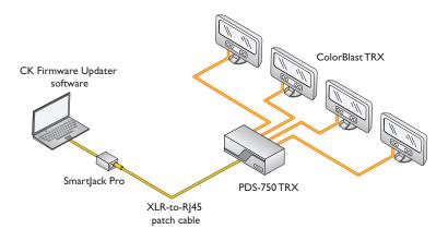
Wou can use an iPlayer 3 controller instead of SmartJack Pro to connect CK Firmware Updater to your lighting network. Connect the DMX 1 output port on iPlayer 3 to the DMX IN port on a PDS-750 TR or PDS-750 TRX with an RJ45-to-female-XLR patch cable, or to the DMX IN port on a PDS-150e or PDS-60 24V using a standard RJ45 patch cable.
