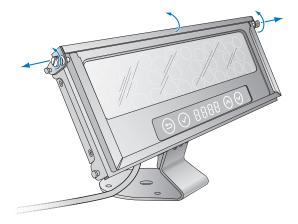
3. Slip the spread lens or accessory into the accessory holder slot.
