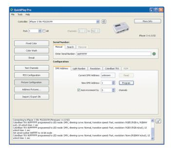
5. To set the fixture's resolution, click the Resolution tab, select 8-bit or 16-bit from the New Resolution drop-down list, and click Program.
