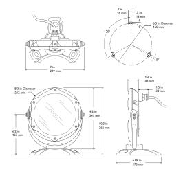
High output, underwater — This submersible fixture offers the full range 16.7 million RGB colors and an output of over 500 lumens.
