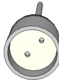
**Open Back Glass Enclosed:** A fixture that encloses the lamp in glass and is open to the air in the back/top of the track head. Variations of this fixture type may have additional metal supports near the sockets or the stem from the track. The glass may be frosted or have a pattern.
